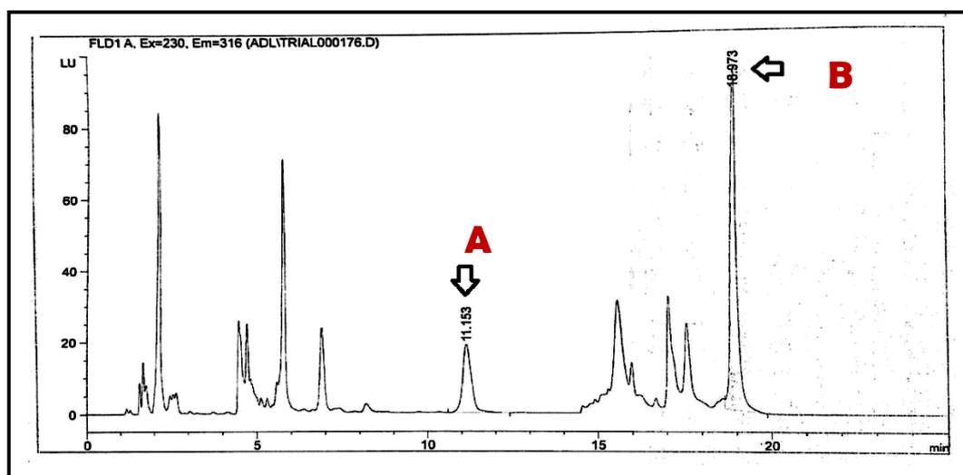
Fig. (3): HPLC chromatogram of BPA in one obese child showing: (A) detectable urinary bisphenol-A level peak at retention time 11.153 minute ( $> \text{LOD}^*$ ), (B) bisphenol-BP internal standard peak at retention time 18.973 minute.
