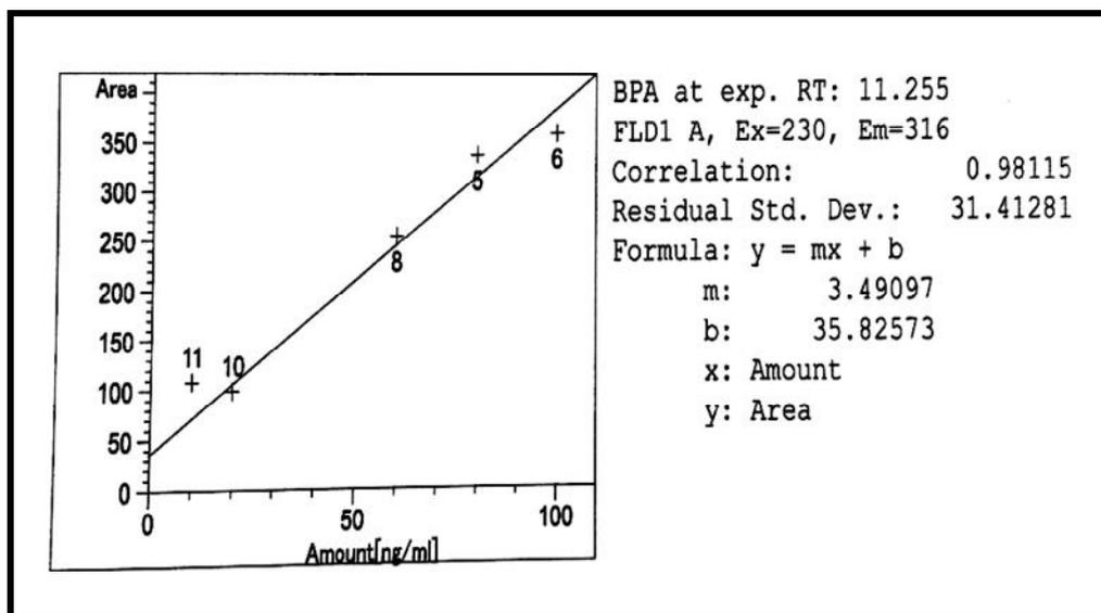
Fig. (2): Bisphenol-A standard calibration curve
